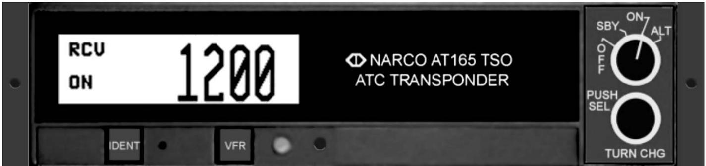
FIGURE 1-1 AT 165 FRONT PANEL
